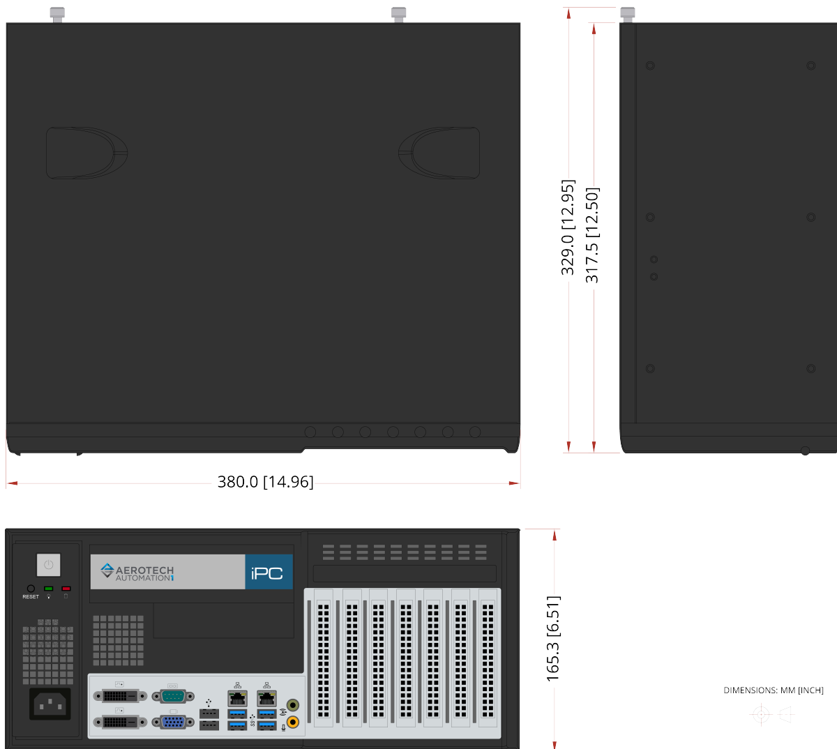
Figure 1-5: Desktop Computer Dimensions (-DT01)
