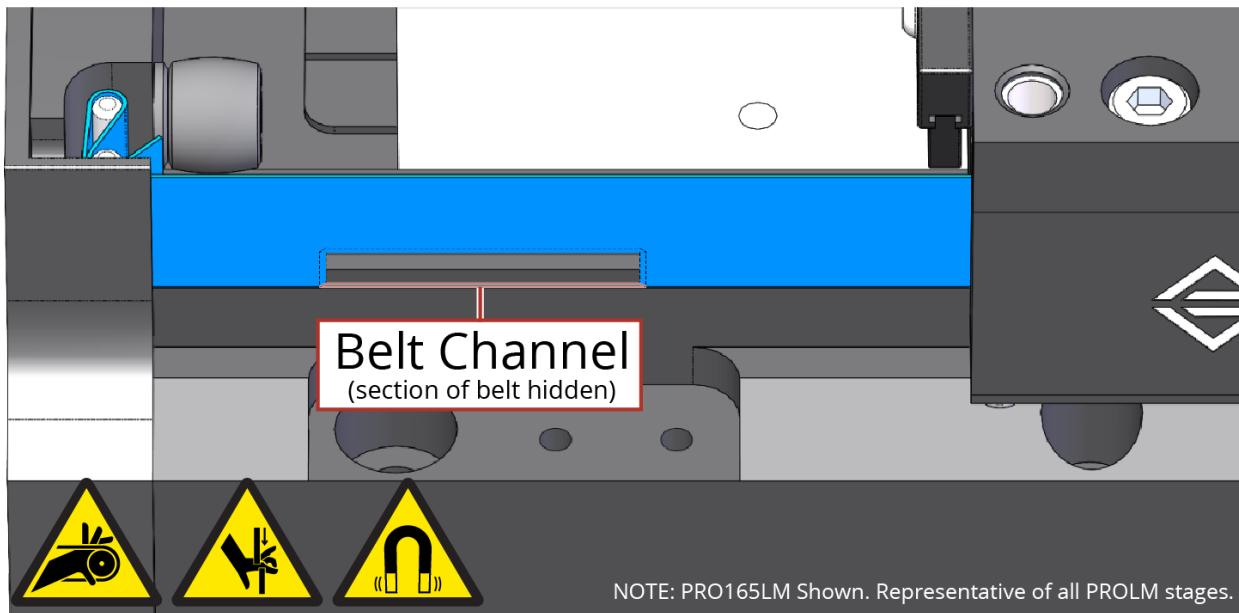
12. Once the belt is fully adjusted, trim the ends of the belt as shown in [Figure 4-11](#).
