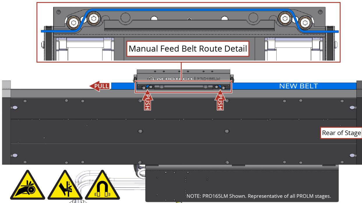
6. Manually pull the new belt back and forth through the table. Confirm that the side seal belt feeds through smoothly without friction or snagging. If there appears to be damages preventing successful installation, contact Aerotech Global Technical Support .
