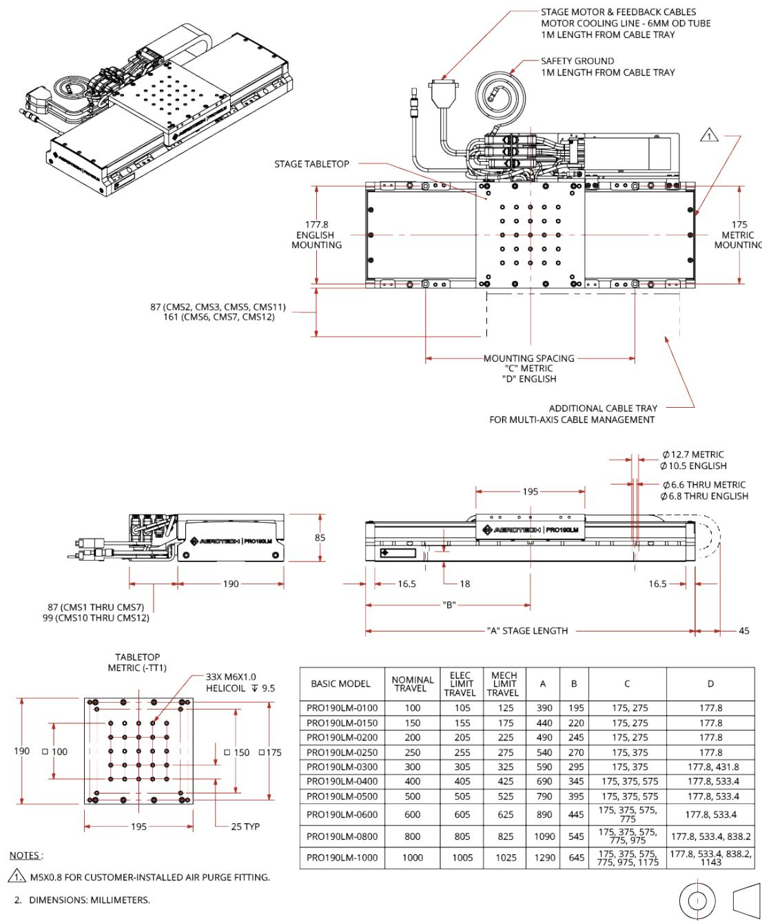
Figure 2-2: PRO190SL Tabletop Dimensions (-TT2/-TT3 Option)
