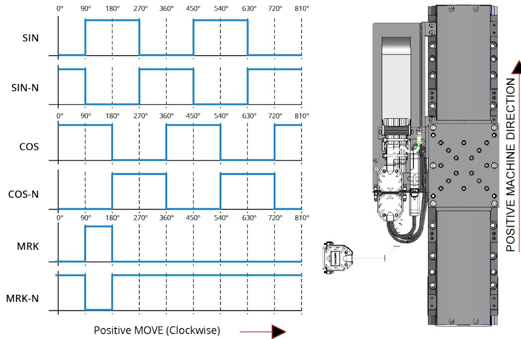
**Figure 3-7: Encoder Phasing Reference Diagram (Sine Wave)**
