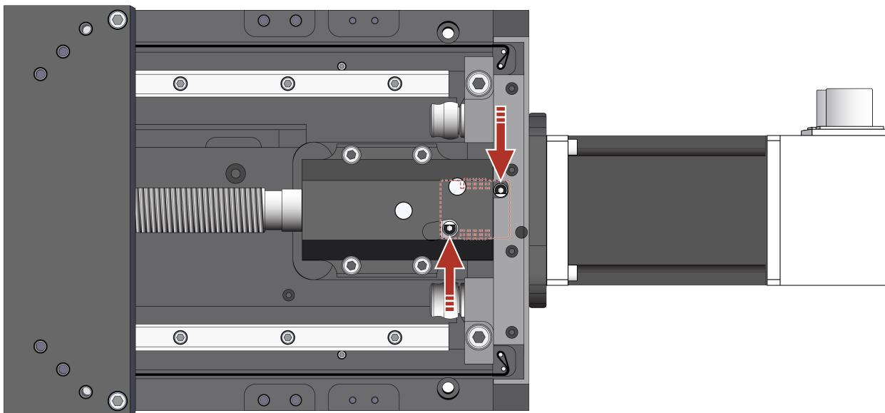
8. Rotate the drive screw by hand to ensure that the drive screw rotates freely.
