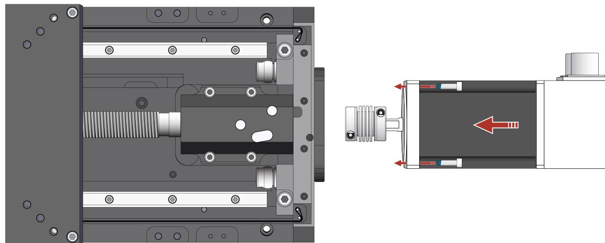
7. Tighten the Shaft Coupling to the drive screw (Figure 4-7). Refer to Table 4-1 for the correct hardware and torque requirements.
