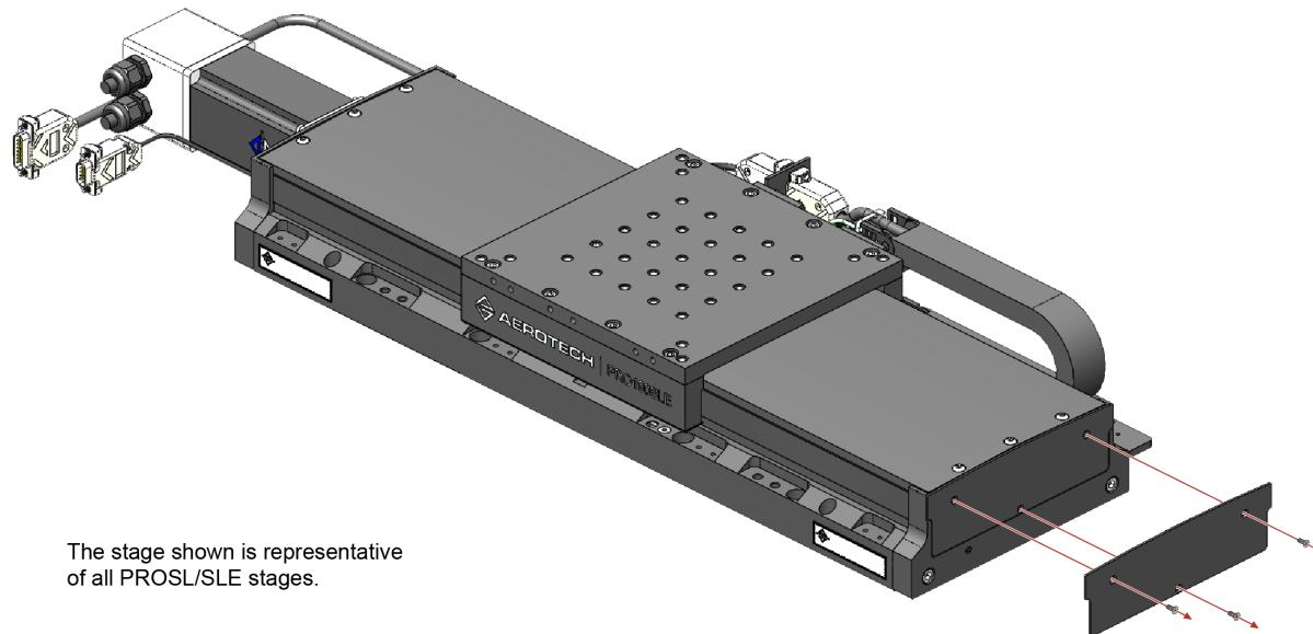
**Figure 4-2: Hardcover Screw Removal**
