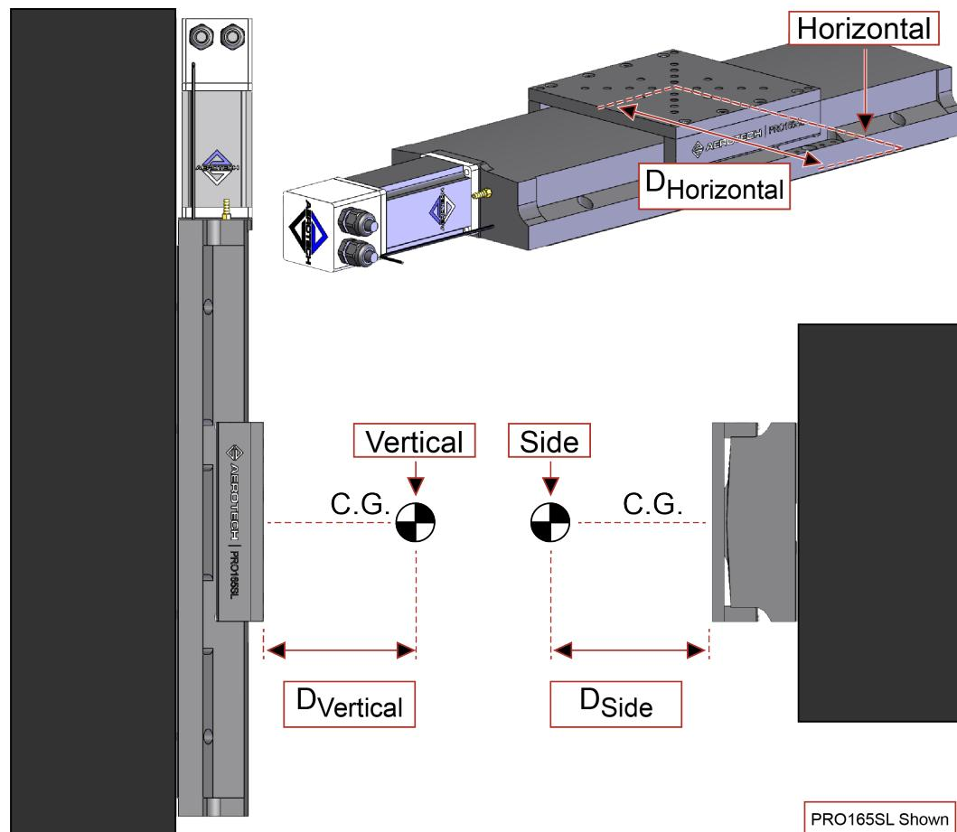
**Figure 2-7: Cantilevered Load Capability**
