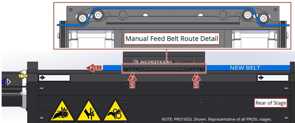
6. Manually pull the new belt back and forth through the table. Confirm that the side seal belt feeds through smoothly without friction or snagging. If there appears to be damages preventing successful installation, contact Aerotech Global Technical Support .
