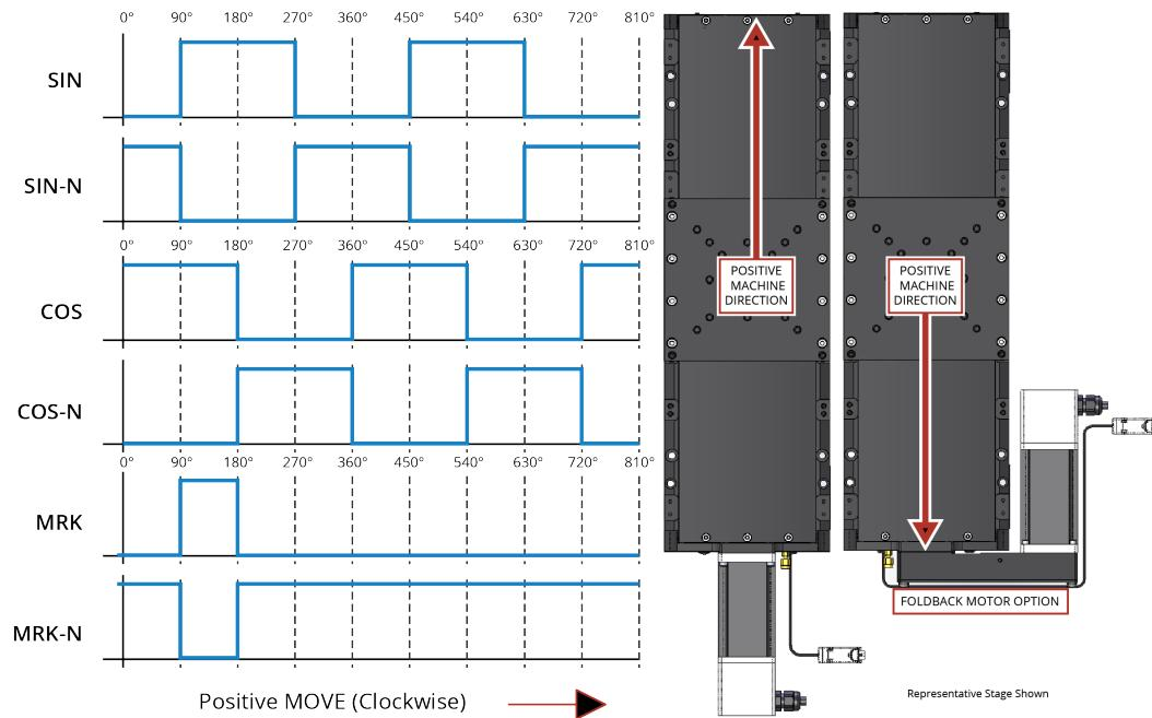
**Figure 3-6: Encoder Phasing Reference Diagram (Sine Wave)**
