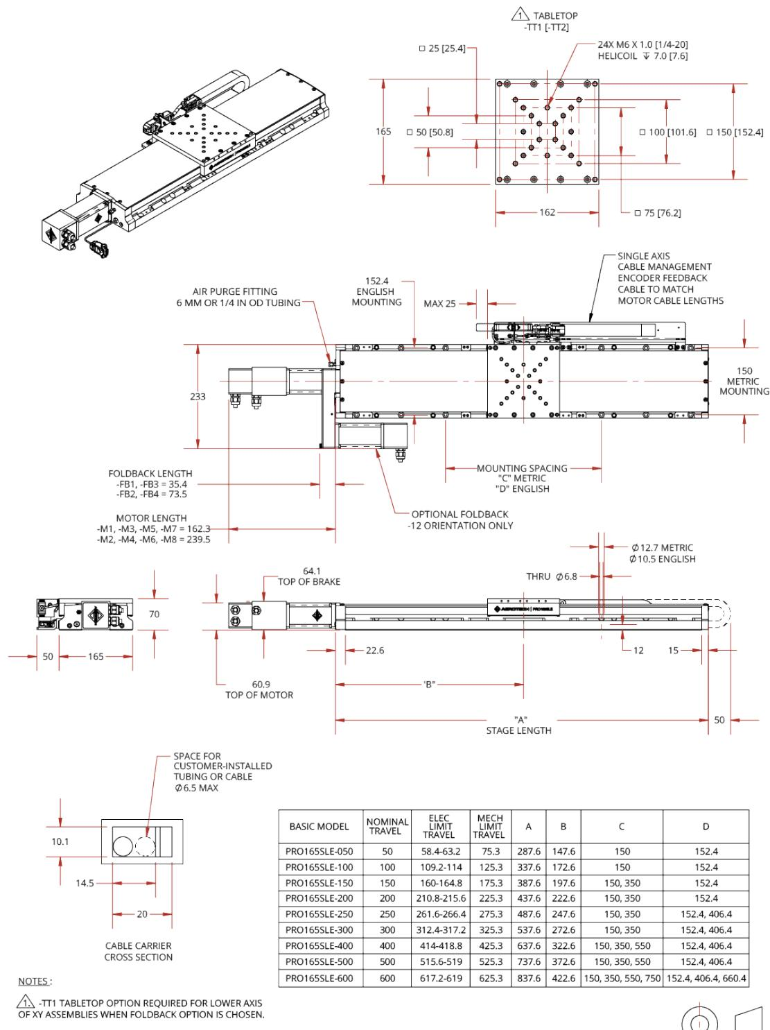
Figure 2-4: PRO165SLE Tabletop Dimensions (-TT3 Option)
