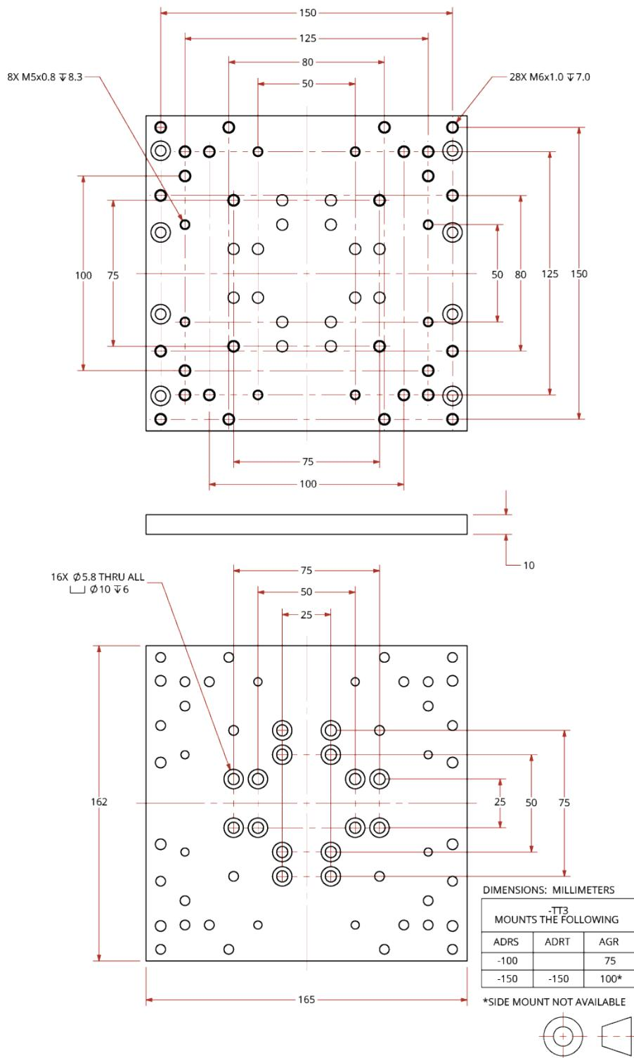
Figure 2-5: Z-Axis Bracket Dimensions
