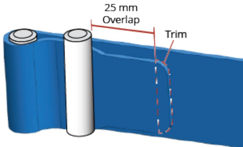
13. Create a permanent loop on both ends of the side seal belt by applying a small amount of super glue (cyanoacrylate glue) to the overlapping end tabs. The belt can be removed from the pins to avoid getting excess glue on stage components.
