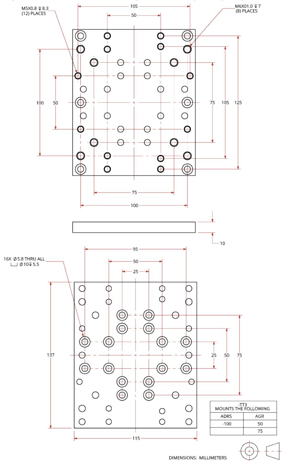
Figure 2-5: Z-Axis Bracket Dimensions
