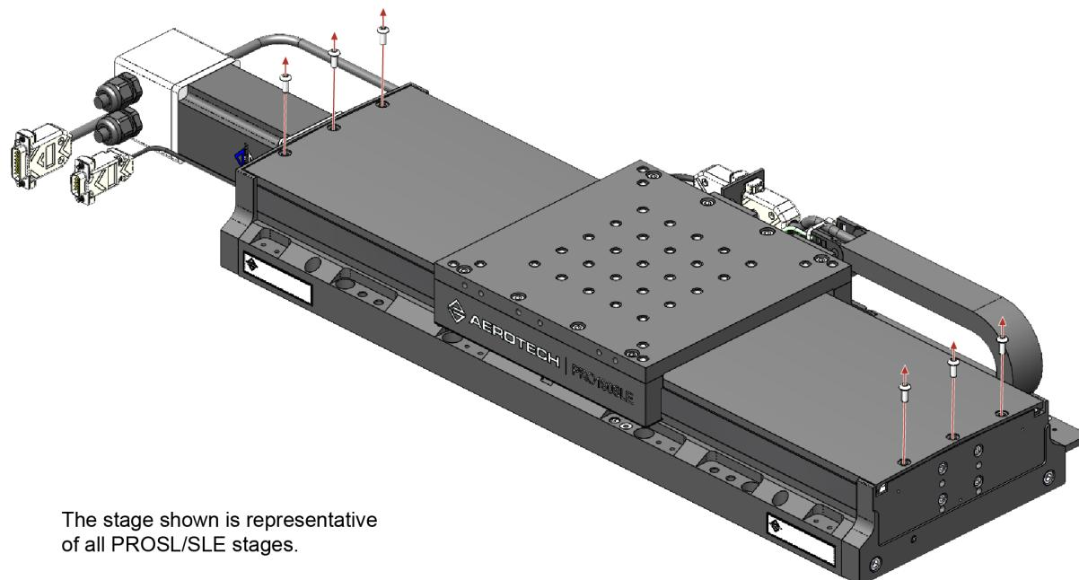
**Figure 4-3: Hardcover Removal**
