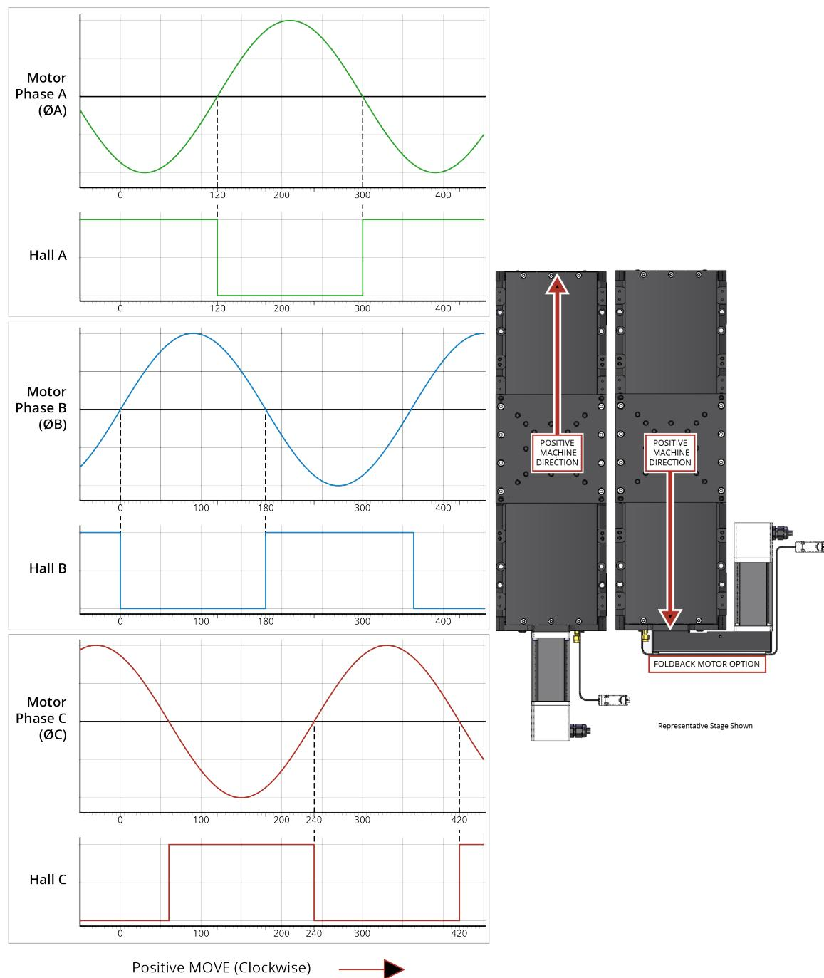
**Figure 3-5: Encoder Phasing Reference Diagram (Standard/Square Wave)**
