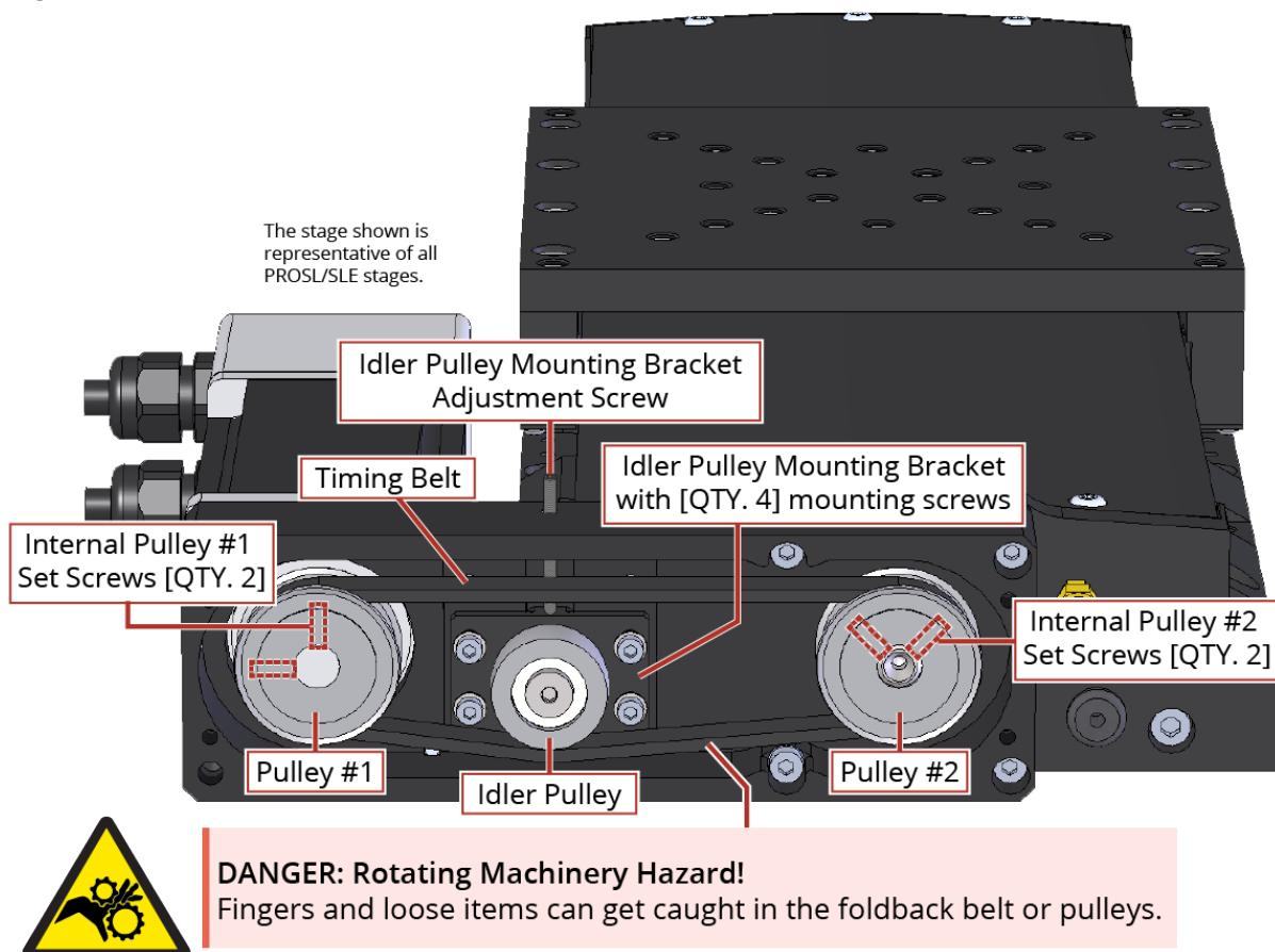
Figure 4-18: Lubricate the Pulley Flanges
