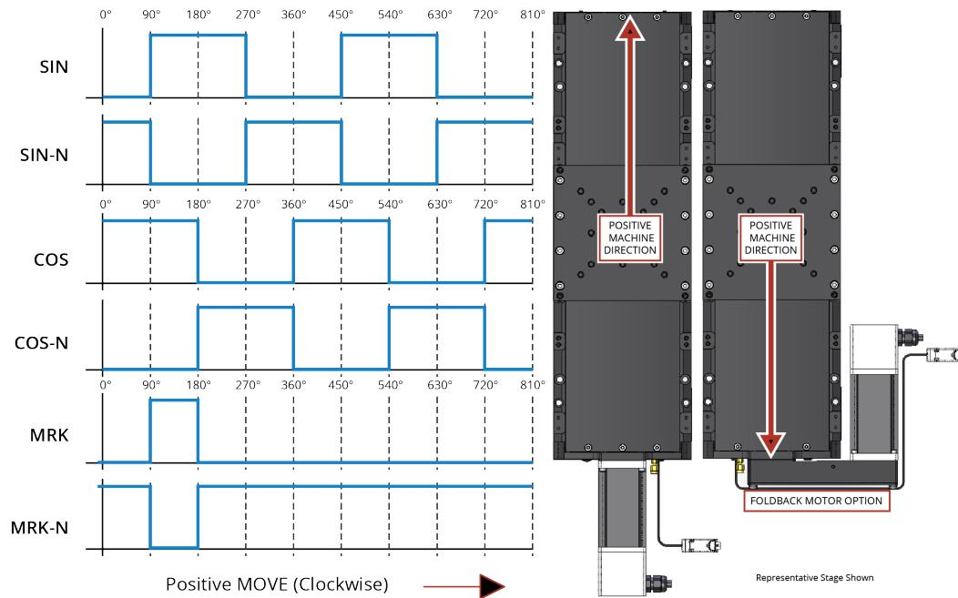
**Figure 3-6: Encoder Phasing Reference Diagram (Sine Wave)**
