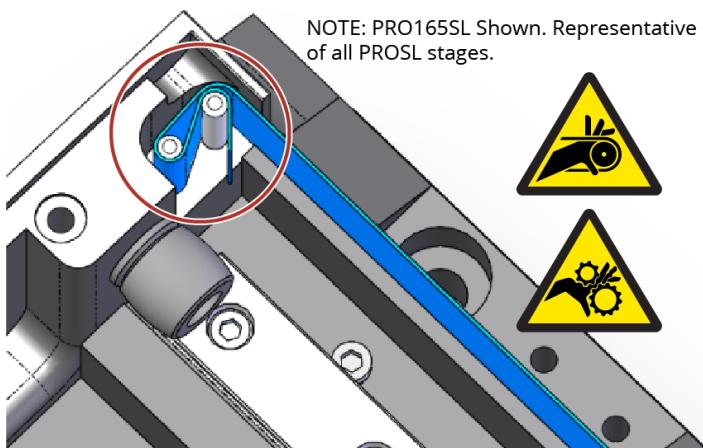
9. Adjust the tension on the left and right sides. Make sure that the spring is centered and stretched. Make sure that there is enough tension in the spring to satisfy all alignment requirements.
