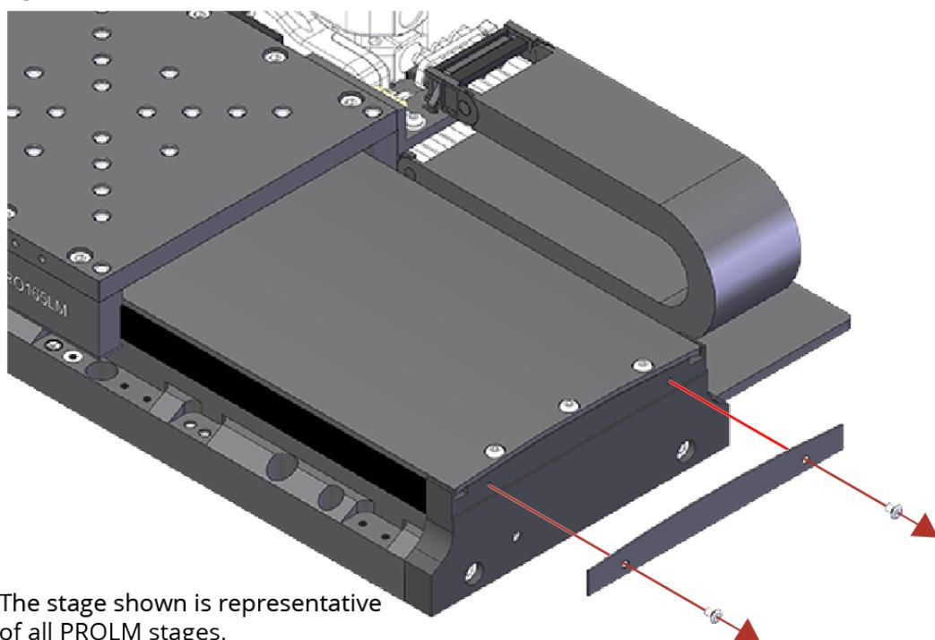
**Figure 4-2: Hardcover Screw Removal**
