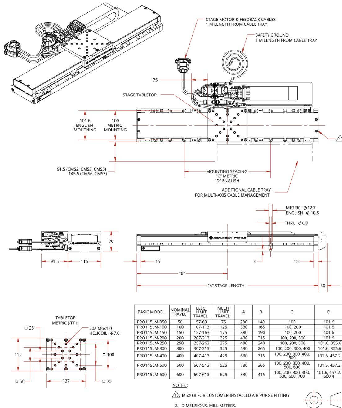
Figure 2-2: PRO115LM Tabletop Dimensions (-TT2/-TT3 Options)
