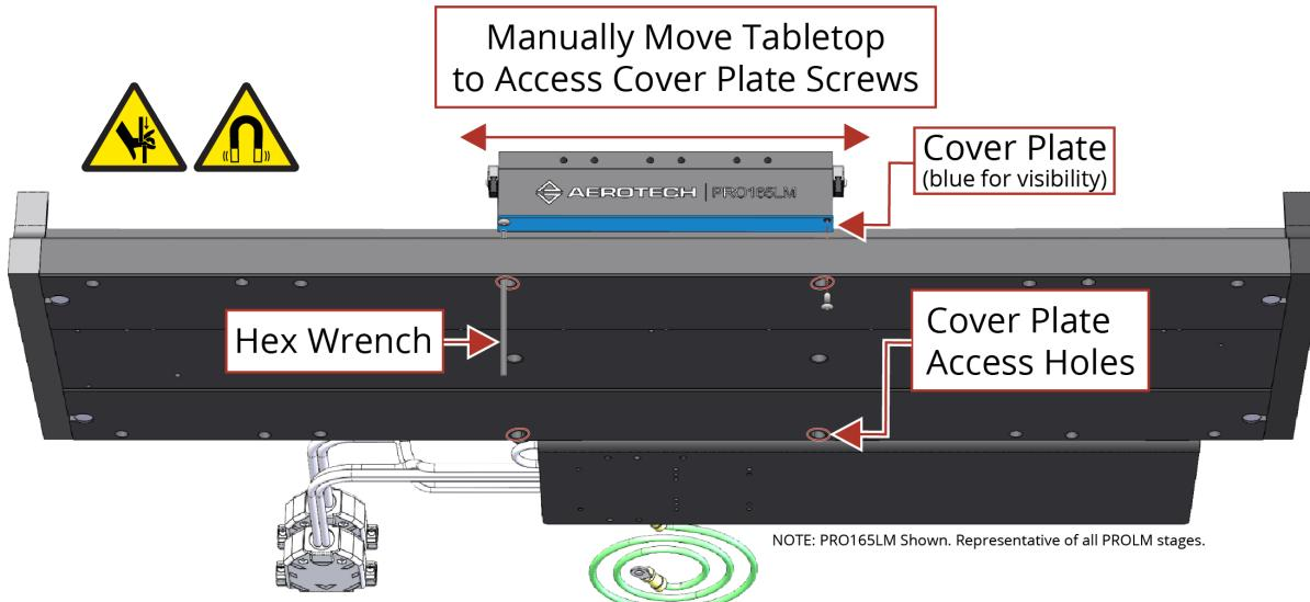
**Figure 4-8: Manual Feed Method**
