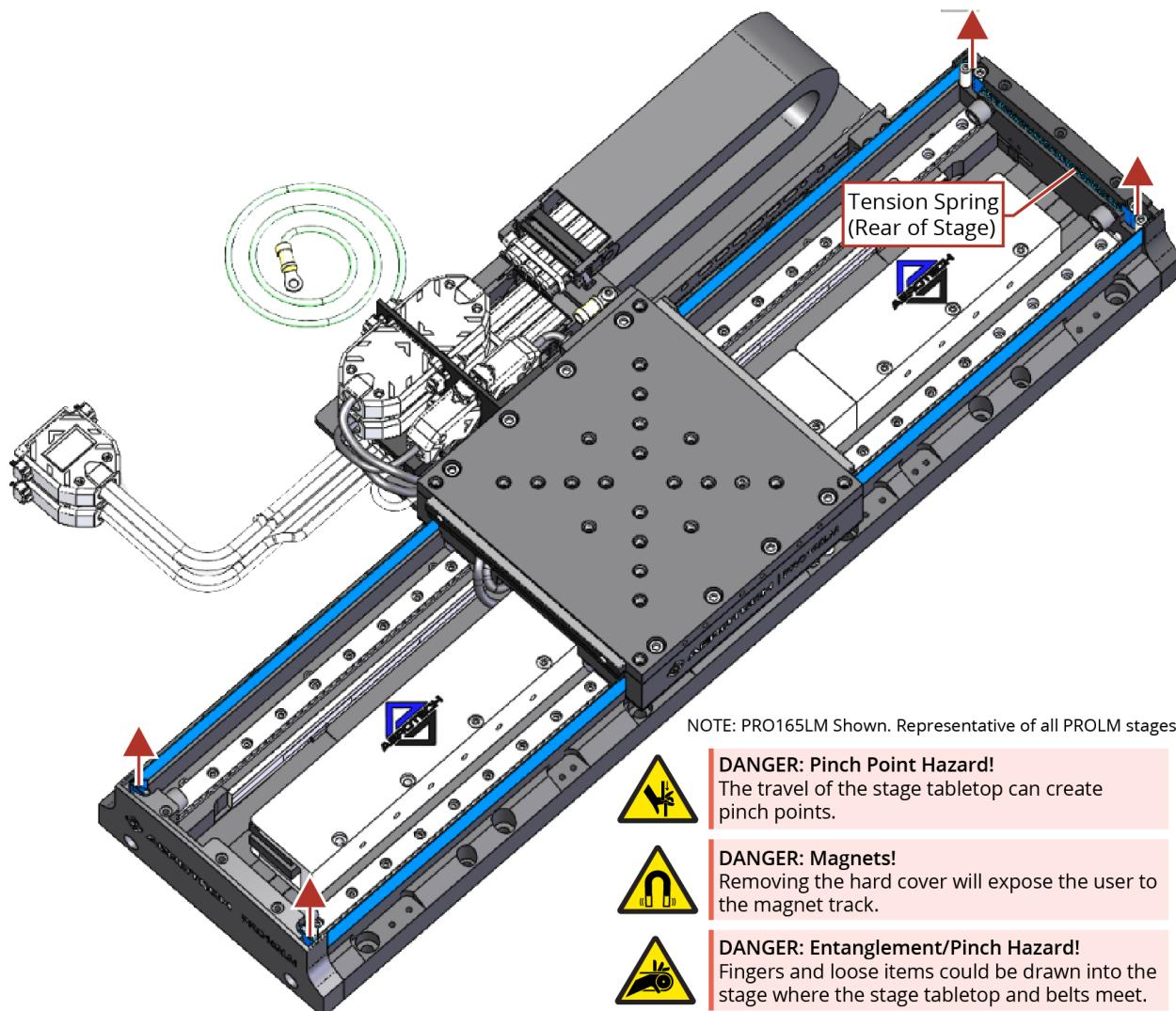
3. Install the new side seal belt at the rear of the stage.
