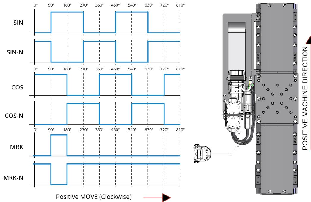
**Figure 3-7: Encoder Phasing Reference Diagram (Sine Wave)**
