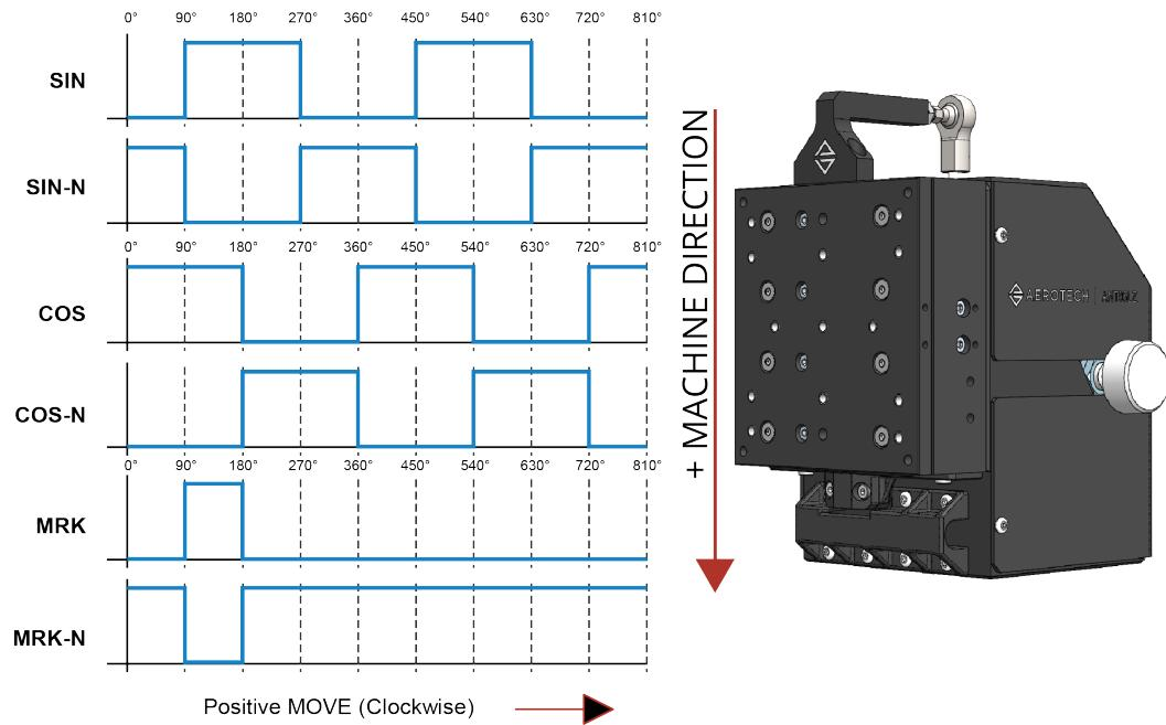
**Figure 3-6: Encoder Phasing Reference Diagram (Sine Wave)**
