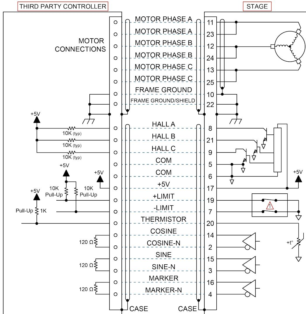
Figure 3-2: ANT95LZ Motor and Feedback Wiring [-E3 Option]
